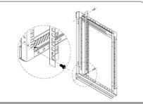
Fix 19" mounting rails to the first holes of top & bottom of side frames by 4sets of M5 screws.
