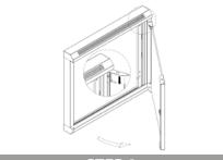
Open the front door by key, pull the door latch downward, refer to the picture, remove the front door from front frame, put them separate for the preparation of the frame assembly.
