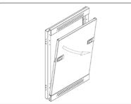
Remove panels from side frames, put them separate for the preparation of the frame assembly.
