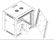
Install the panels and front door as showed in the picture. Adjust the diagonal size so door can work well.
