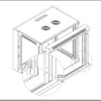
Install front frame by 4pcs of M6\*12 screws (6pcs of M6\*12 screws if more than 18U), refer to the picture.
