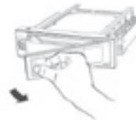
2. Place the hard drive into HDD-ROM with the hard drive label (printed) side up and be sure the hard disk Connectors side is inserted into HDD-ROM.
