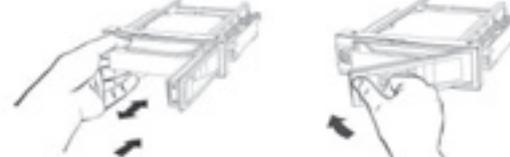
The front panel door will not be closed firmly if hard disk is being inserted in wrong direction. HDD-ROM will get damaged if closed by force.
