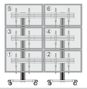
Note: The displays are installed by the numerical order given.
